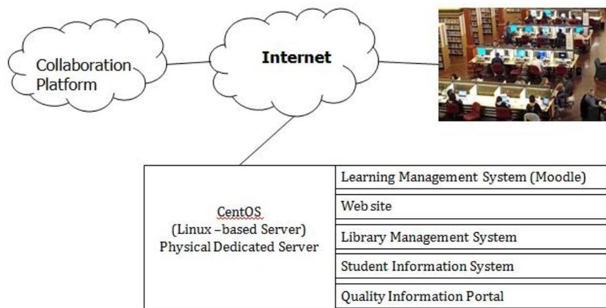
Figure 2. Linux based dedicated server is used as a cloud hosting solution.
